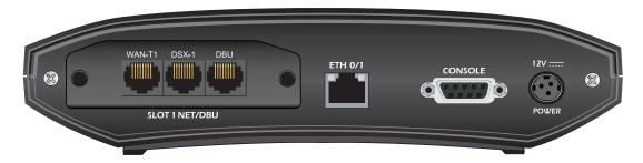
Figure 2. NetVanta 3200 Rear Panel Layout
